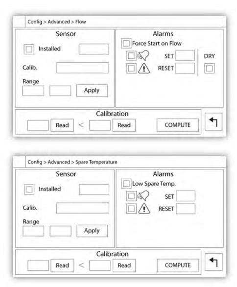
In the ViZiTouch, all sensors refer to analog input connectors on the I/O board. They all have similar settings and configuration.
