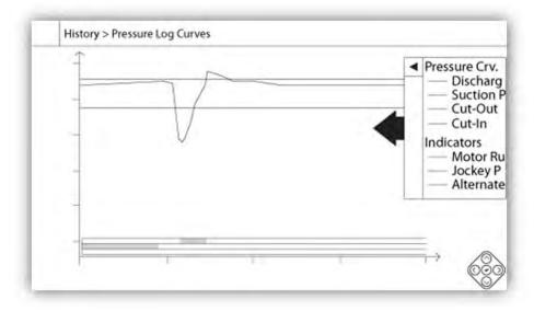
The vertical axis represents the pressure in the actual unit selected. Its scale is dynamic and will resize depending on
