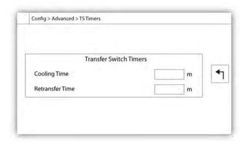
Most common timers for the transfer switch control can be configured here. Note that any timer set to 0 will remove the delay in the decision process.
