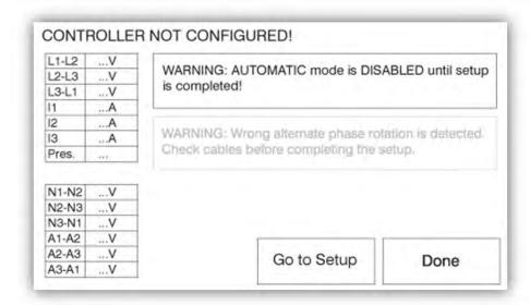
The first Setup must be done prior to using the controller. Completing the First Setup is the only way to access the homepage and enable the automatic mode of the controller.
