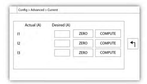
To calibrate a particular current sensing element, enter the current value as read from a calibrated meter and then press compute. For best results, press the ZERO button when no current is flowing through the sensing element before calibrating.
