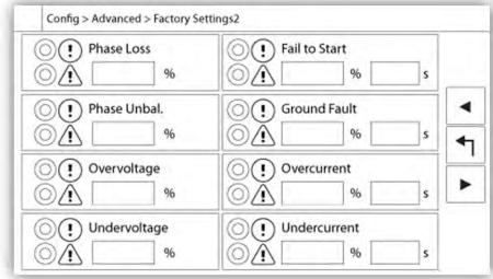
The factory settings are always pre-configured at the factory and set the main parameters of the controller. Most of the settings found on this page can only be changed by an authorized Tornatech employee and is protected by a level 8 password.
