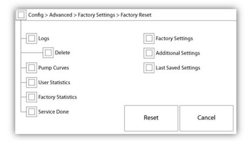
This page will reset the ViZiTouch to the original factory configuration, thus clearing all subsequent configurations performed during the life of the controller.
