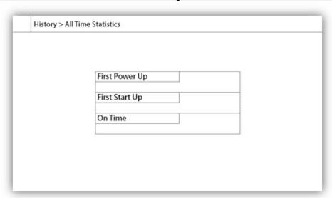
All statistics shown here are calculated since the controller's first start-up was done. All dates are in the YYYY.MM.DD format and all time references are in the HH:MM:SS format.
