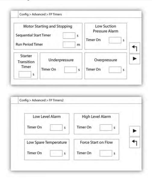
Most common timers can be configured here. Note that any timer set to 0 will remove the delay in the decision process.
