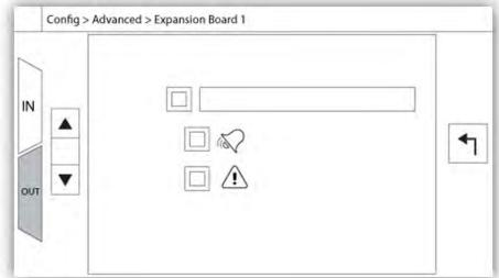
This page allows the configuration of both programmable inputs and outputs available on an IO Expansion board. Two buttons located far left swap between the input and output section of the page. Just beside, two square buttons labelled "+" and "-" are separated by a number that indicates the actual selected input/output. By using the "+ / -" buttons, it is possible to navigate between them easily.
